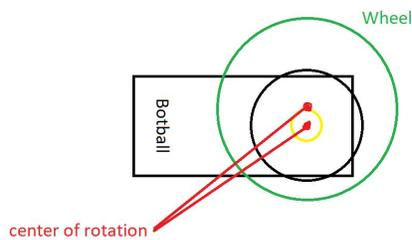
VEX motors have female square hole outputs that accommodate the standard  $\frac{1}{8}$ " shaft size (and  $\frac{1}{4}$ " high strength shaft size on the new V5 motors). As a result, any shafts attached to the motors are concentric and wheels on those shafts are concentric to the motor output as well.
